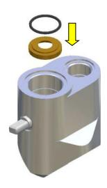
6. Torque end cap to 60Nm.
