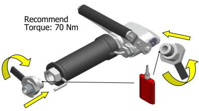
3. Attach vent fitting and tighten to manufacturers instructions.
