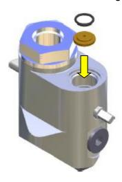
12. Torque vent end cap to 35Nm.
