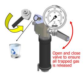
3. Remove fill-side nut & handle assembly.
