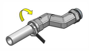
3. Apply anti seize to male thread and insert connection.
